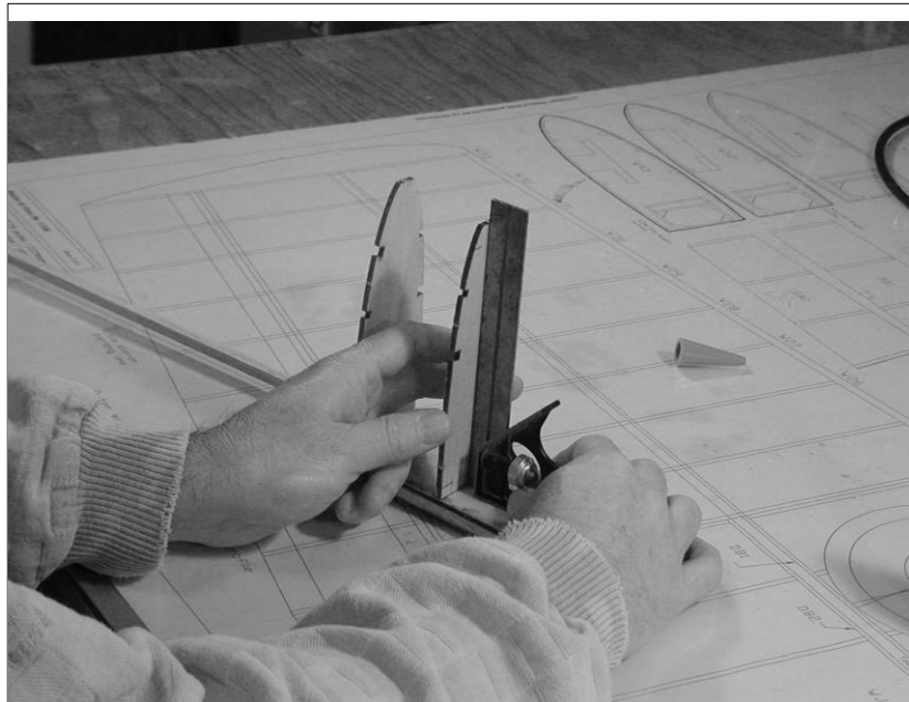
Figure 27: Gluing Ribs to DB1
