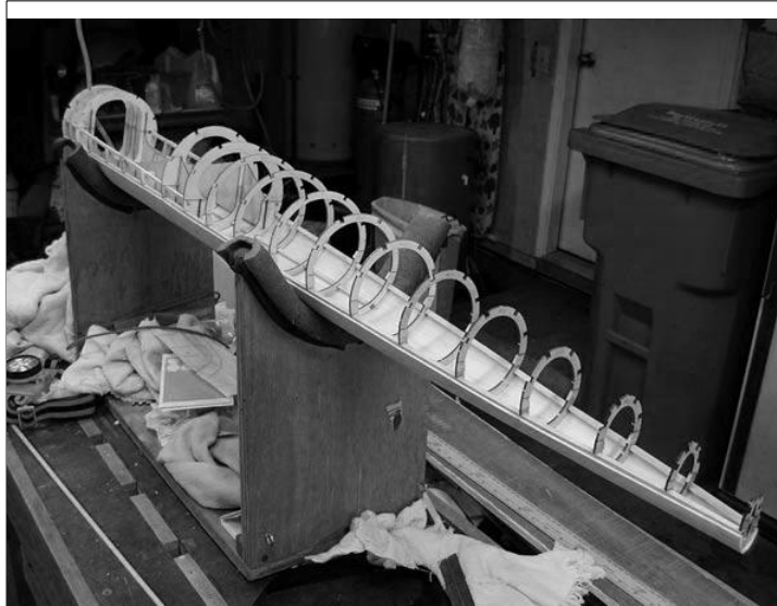
Figure 5: Lower fuse frame-up
