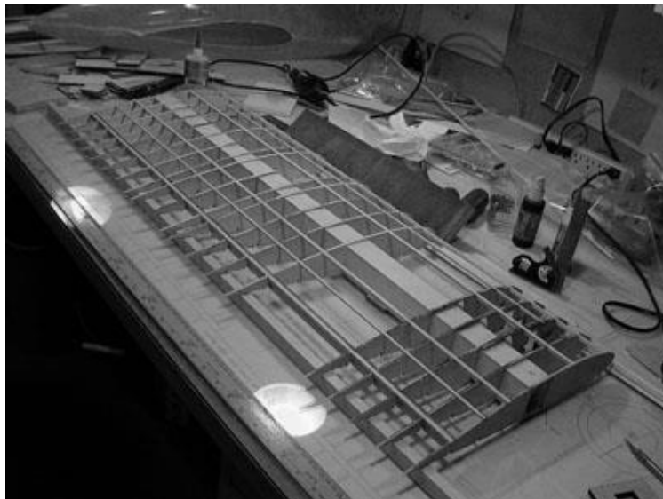
Figure 10: Stringer and Rear Spar Installation
