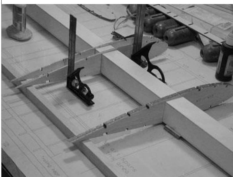
Figure 9: Attaching Ribs to Box Spar
