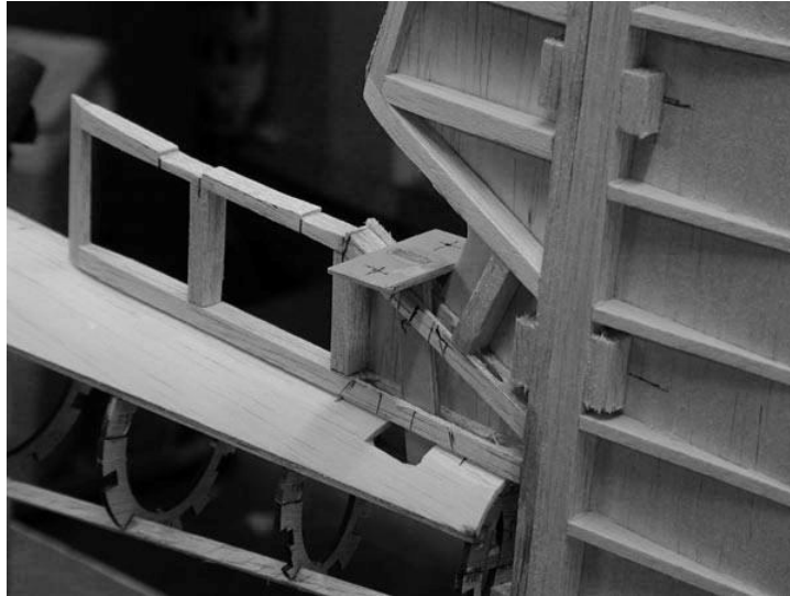
Figure 15: Elevator horn detail
