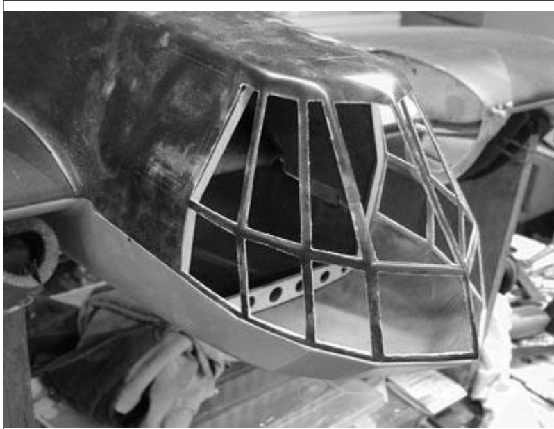
Figure 34: Cutting out the Nacelle Windows
